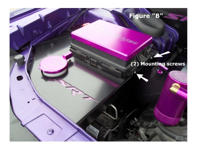
For vehicles equipped with the 3.6 Pentastar engine the (2) Mounting screws are not required as shown in (figure "B"). Use the existing factory extended nut as shown in (figure "C"). Remove the factory extended nut place the ABS cover into position and secure it by replacing the factory extended nut.
