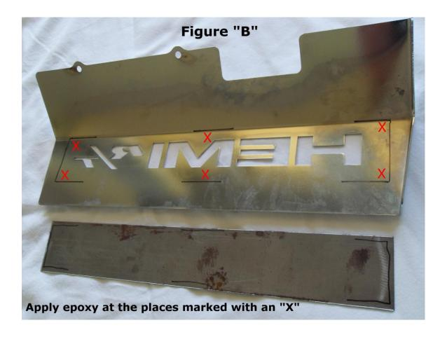
On larger backer plates also include the top and bottom of the plate on center as also shown in figure "B".
