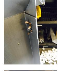
2. Place one washer on a bolt, then insert it through the Plexiglass and top, use a acorn nut to tighten from the backside of the stand. Repeat process for all 4 corners
