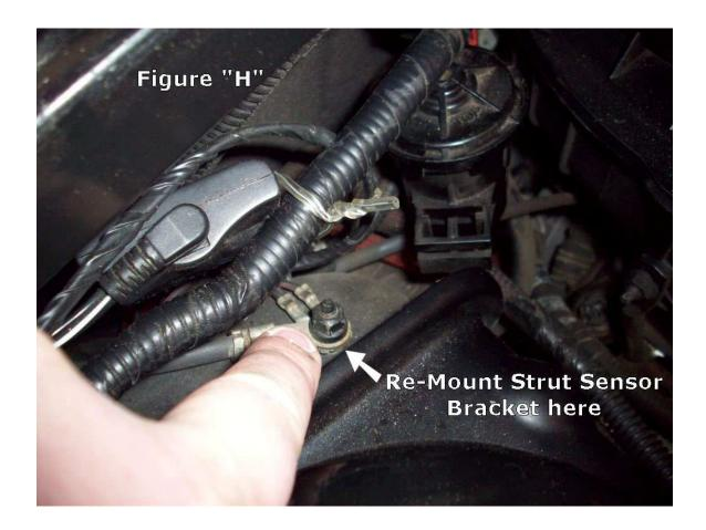
Remove the nut and then the (3) ground wires then put the bracket on first then the (3) ground wires them turn the purge solenoid towards the back of the car and secure them all in place with the nut as shown in figure "I".
