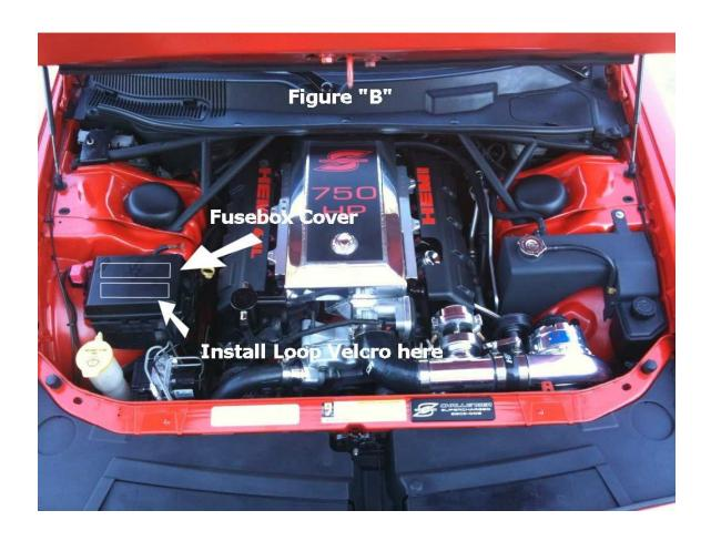
Once the installation is complete the final position of the cover should look like the picture as shown in figure "C".
